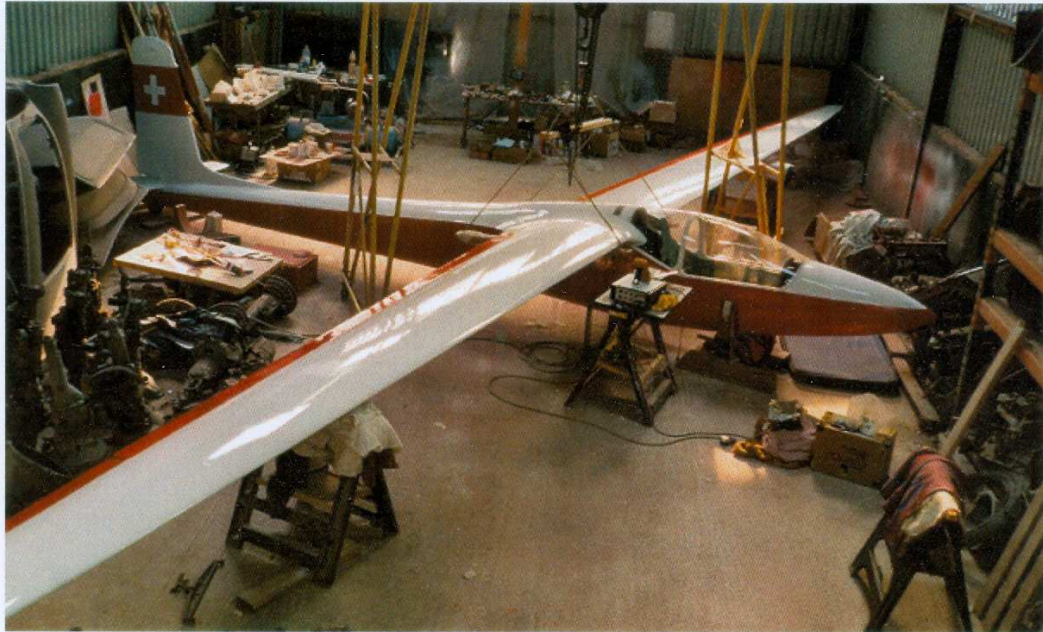
Fig. 5.13 Assembly for weighing after painting
