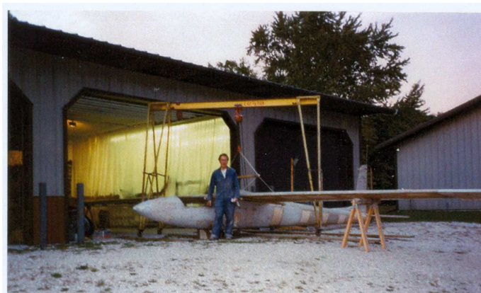
Fig. 3.11 First assembly to check controls
