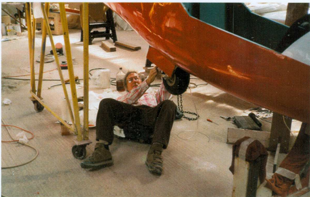
Fig. 5.14 Adding hydraulic fluid to suspension
