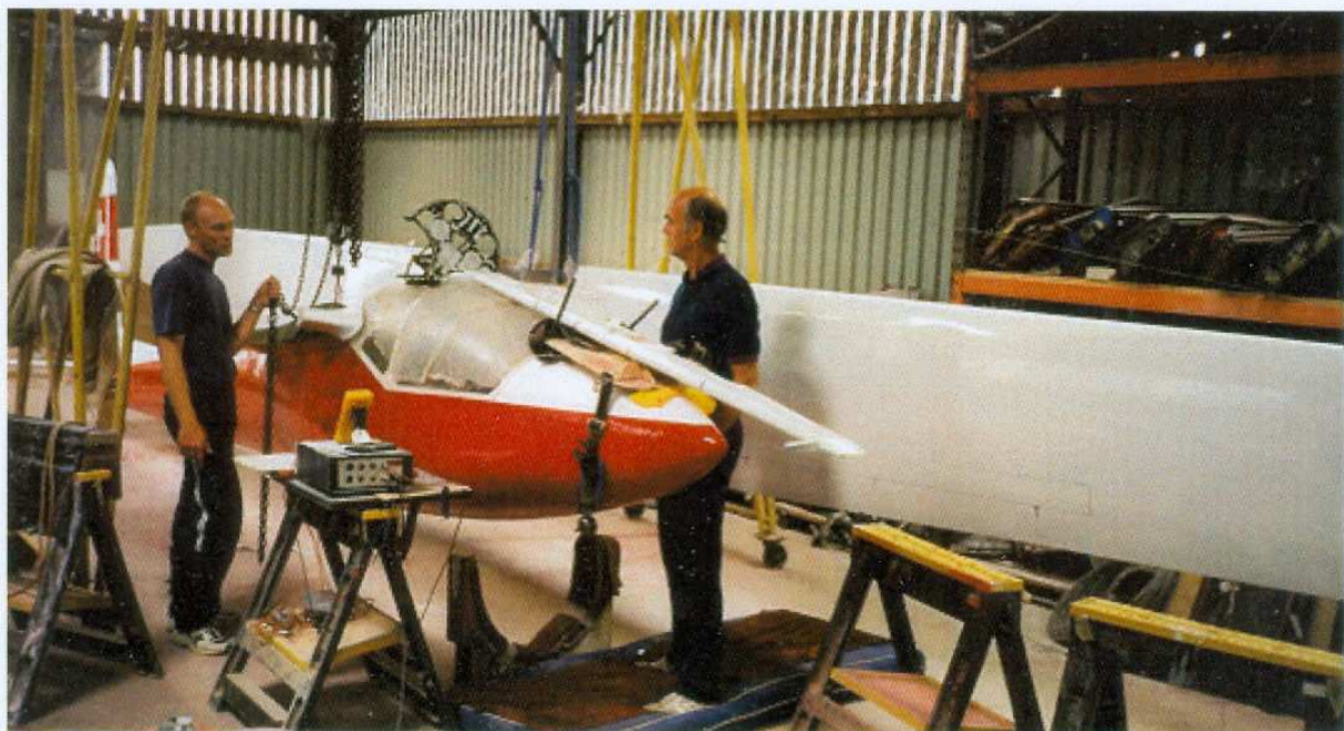
Fig. 5.12 Weighing after painting
